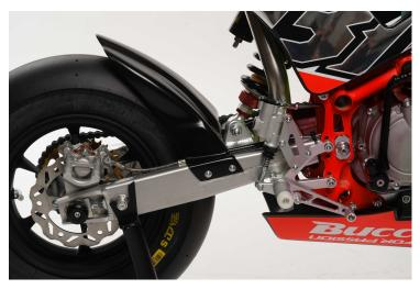
**Frame** Steel trellis frame, 3D CAD designed with round and oval high strength
